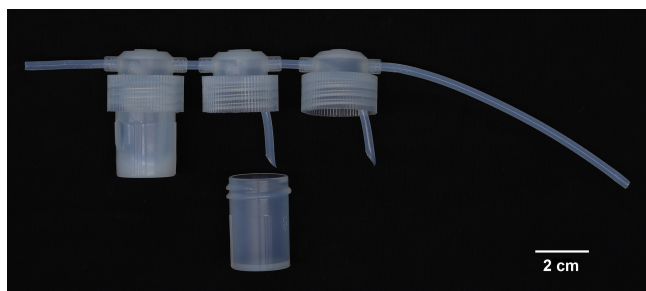
Figure 4. PFA transfer closures connected in sequence for the last 3 of 10 flat bottom PFA vials as shown in Fig. 5.
